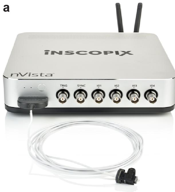
**Fig. 2.** Next-generation miniscope. Control and data-acquisition device for the Inscopix nVista miniscope system allowing remote control via a web-browser-enabled GUI.
